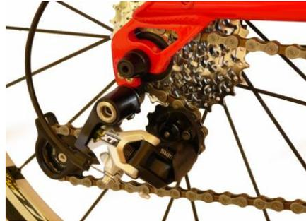
1. Shift onto the smallest chainring in the front and shift down to the smallest cog in the rear
