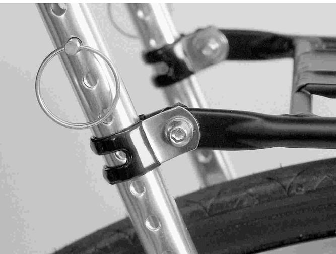
The recline of the seat is determined by the position of the pins in the telescoping seat support tubes; these are located on the back of the seat. To adjust the recline of the seat, simply pull the pins, adjust up or down, and replace the pins. Remember to be sure each pin is pushed in completely after making any adjustment.
