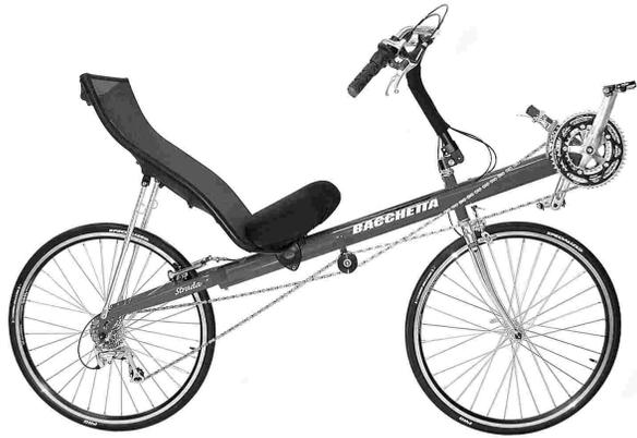
The derailleurs function is to push the chain sideways from one chainring or cog to the next. Derailleurs are connected to the shifters by cables. The shifter pulls the moving part of the derailer sideways; a spring pulls it back when the shifter is turned the other way.
