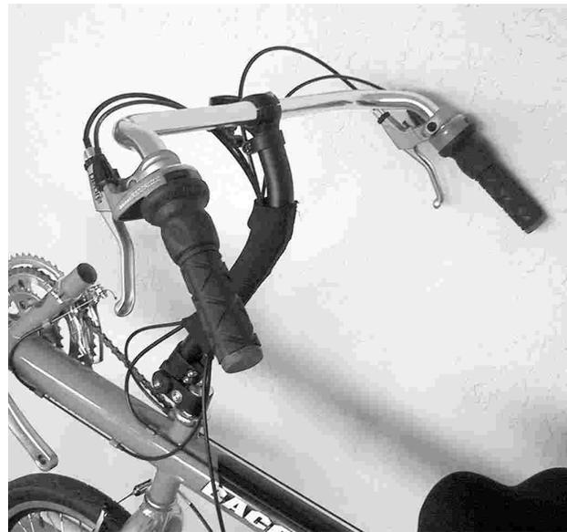
parallel with the ground when viewed from one side. Once the riser is secured by the riser clamp located on the bottom of the riser, you will need to adjust the handle bars to the correct angle.
